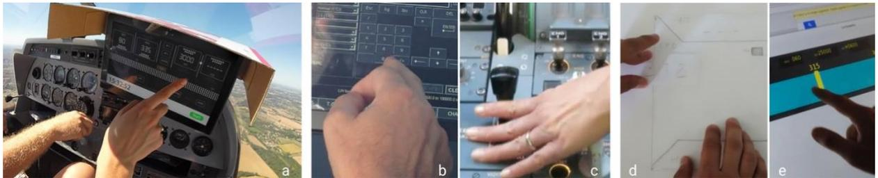
Fig. 1. a) The touch-based flight control panel prototype tested during a real flight (DR400) in unstable weather conditions ; b) an A320 pilot using a touch-based screen for a mission management task ; c) stabilizing the fingers before an action (flaps in an A320 cockpit) ; d) paper-based prototyping with a pilot ; e) walkthrough of the first implementation with a pilot.
